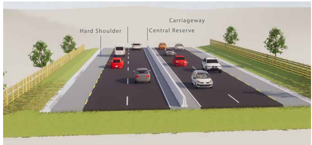
NTS 15: Standard Dual Carriageway Motorway (3 Lane Urban)
