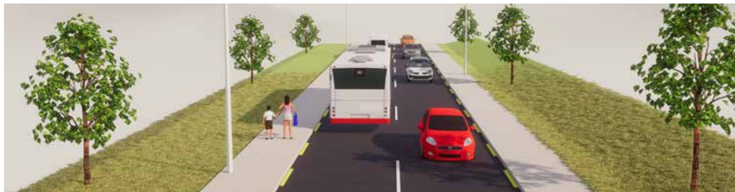
NTS 12: Single Carriageway (With Footway)
