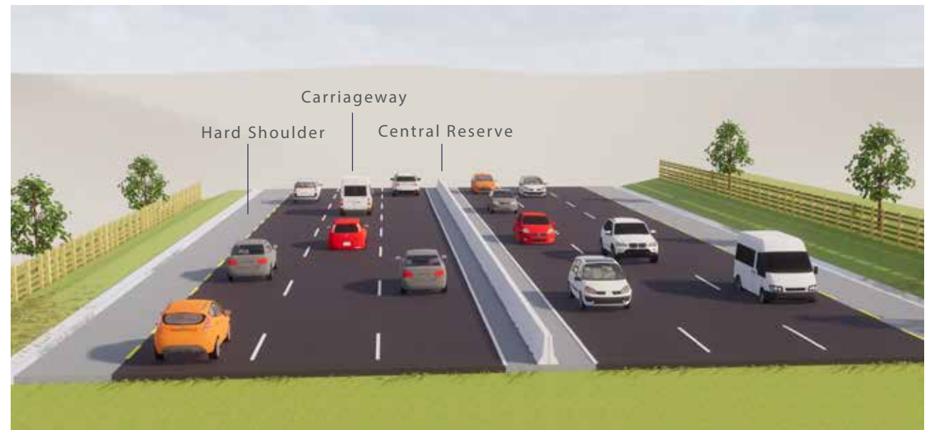
NTS 15: Standard Dual Carriageway Motorway (3 Lane Urban)
